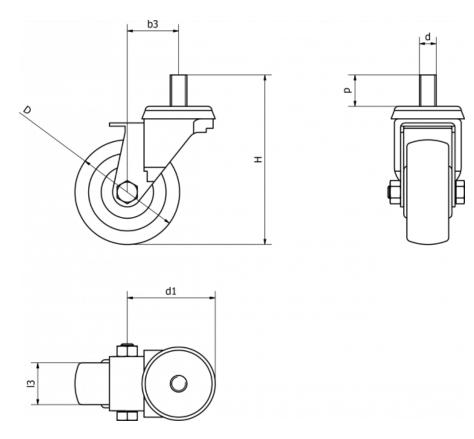
= 59 В Н b3 = 24 L = Code = 18 = 452146 13 = M8= 15 d р D = 40 S = Type = RE.C7-040-CBLd1 = 35 Dynamic load (N) = 300g = 130
